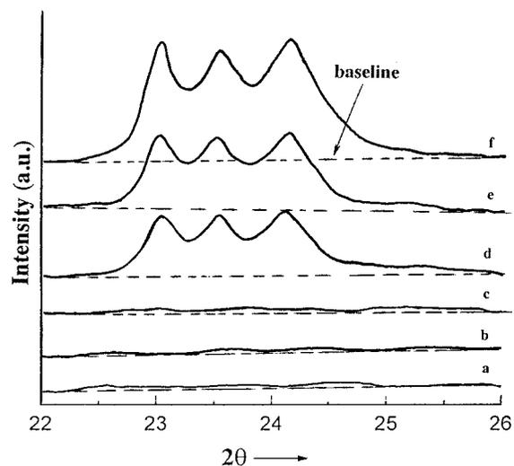
**Figure 1.** XRD patterns: (a)  $\text{CeO}_2$ ; (b, c, and d)  $\text{WO}_3/\text{CeO}_2$  samples with  $\text{WO}_3$  loading of 1.2, 4.0, and 6.0  $\text{W}^{6+}$  ions  $\text{nm}^{-2}(\text{CeO}_2)$ , respectively; (e) a mechanical mixture of  $\text{WO}_3$  and  $\text{CeO}_2$  (3.0  $\text{W}^{6+}$  ions  $\text{nm}^{-2}(\text{CeO}_2)$ ); (f)  $\text{WO}_3$ .
