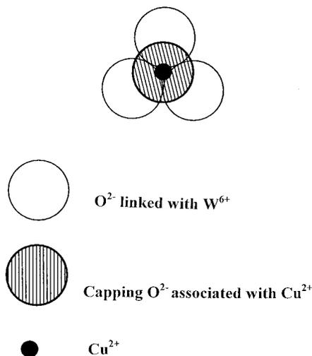
**Figure 12.** A tentative model of "surface tetrahedrally coordinated  $\text{Cu}^{2+}$  species" formed on a  $\text{CeO}_2$  support premodified with a close-packed monolayer of  $\text{WO}_3$ .
