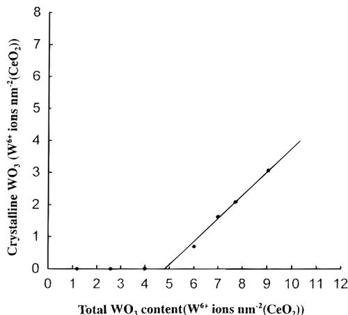
**Figure 2.** Amount of crystalline  $\text{WO}_3$  measured by XRD quantitative analysis versus tungsten oxide content in  $\text{WO}_3/\text{CeO}_2$  samples.
