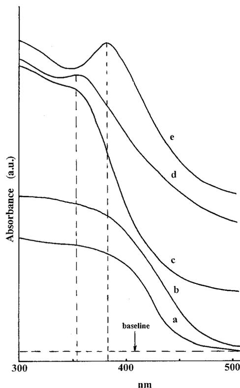
**Figure 7.** UV-DRS profiles of various samples: (a)  $\text{CeO}_2$ ; (b)  $\text{WO}_3$ ; and  $\text{WO}_3/\text{CeO}_2$  samples with various  $\text{WO}_3$  loadings ( $\text{W}^{6+}$  ions  $\text{nm}^{-2}(\text{CeO}_2)$ ) (c) 1.2; (d) 2.0, and (e) 4.6.
