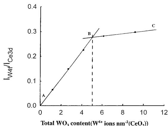
**Figure 4.** XPS peak intensity ratio  $I_{\text{W}4f}/I_{\text{Ce}3d}$  versus tungsten content in  $\text{WO}_3/\text{CeO}_2$  samples.
