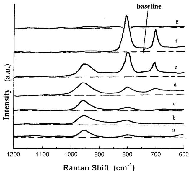
**Figure 5.** Raman spectra of  $\text{WO}_3/\text{CeO}_2$  samples with various  $\text{WO}_3$  loadings ( $\text{W}^{6+}$  ions  $\text{nm}^{-2}(\text{CeO}_2)$ ): (a) 1.2; (b) 2.0; (c) 3.2; (d) 5.0; (e) 9.0; and spectra of  $\text{WO}_3$  (f) and  $\text{CeO}_2$  (g).
