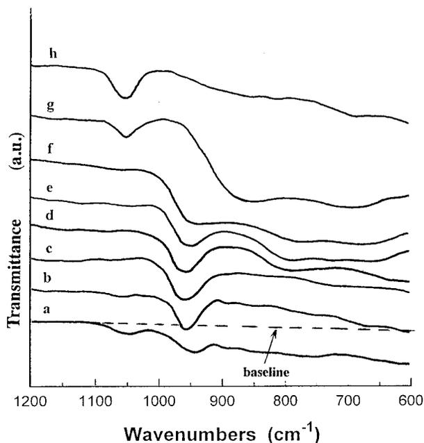
**Figure 6.** Infrared spectra of  $\text{WO}_3/\text{CeO}_2$  samples with various  $\text{WO}_3$  loadings ( $\text{W}^{6+}$  ions  $\text{nm}^{-2}(\text{CeO}_2)$ ): (a) 1.2; (b) 2.0; (c) 3.2; (d) 5.0; (e) 7.2; (f) 9.0; and spectra of a mechanical mixture of  $\text{WO}_3$  and  $\text{CeO}_2$  (3.0  $\text{W}^{6+}$  ions  $\text{nm}^{-2}(\text{CeO}_2)$ ) (g) and  $\text{CeO}_2$  (h).
