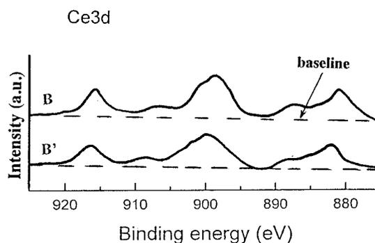
**Figure 3.** XPS spectra: A, A' and B, B' are  $\text{W}4f_{5/2,7/2}$  and  $\text{Ce}3d$  spectra of a  $\text{WO}_3/\text{CeO}_2$  (with  $\text{WO}_3$  loading of  $4.0\text{W}^{6+} \text{ ions nm}^{-2}(\text{CeO}_2)$ ) and  $\text{WO}_3$  and  $\text{CeO}_2$  samples, respectively.
