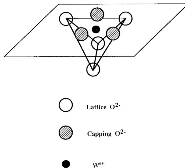
**Figure 9.** A tentative model of the surface tungsten oxide species formed on the (111) plane of  $\text{CeO}_2$  support.
